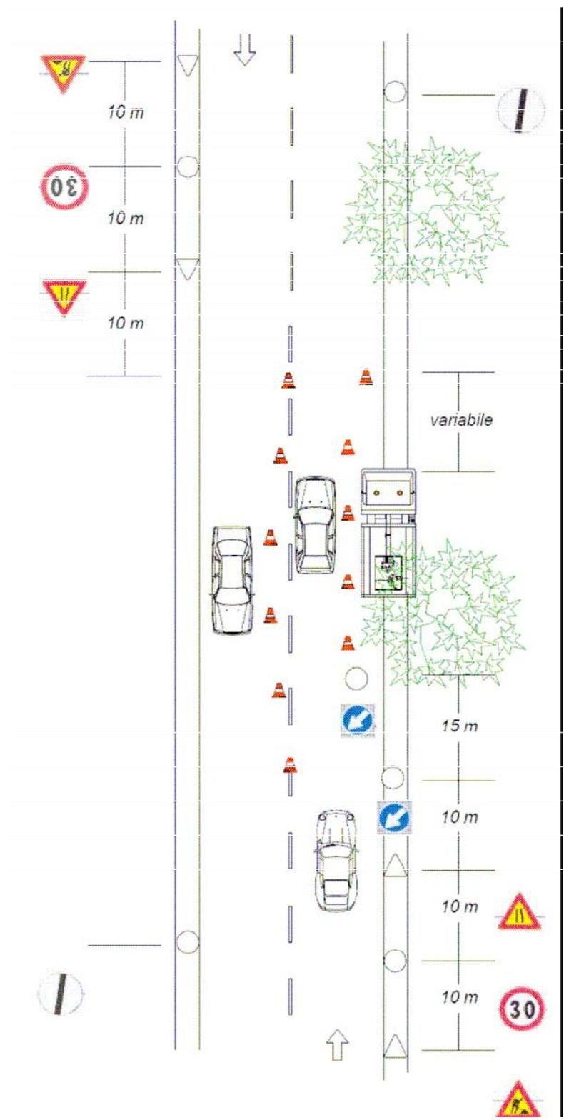
INSTALLAZIONE DI CANTIERE TEMPORANEO – ALLEGATO 6 - CANTIERE URBANO A MARGINE DELLA CARREGGIATA IN PROSSIMITÀ DI INCROCIO
